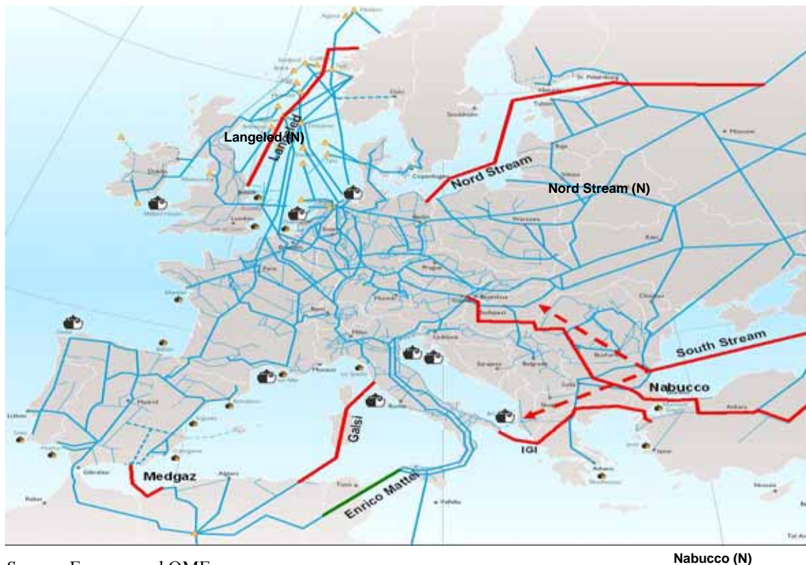
Figure 3. Import pipelines to Europe, projects and reinforcements, 2008
